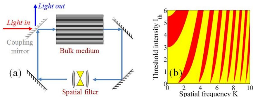
**Figure 1.** (a) Schematic diagram of an optical ring cavity filled with a bulk nonlinear (e.g., Kerr) material so that light-medium interactions can take place over a finite propagation length. (b) Typical multi-Turing threshold instability curves for the thin-slice cavity system [4]. The introduction of finite medium length changes some key characteristics of the spectrum.
