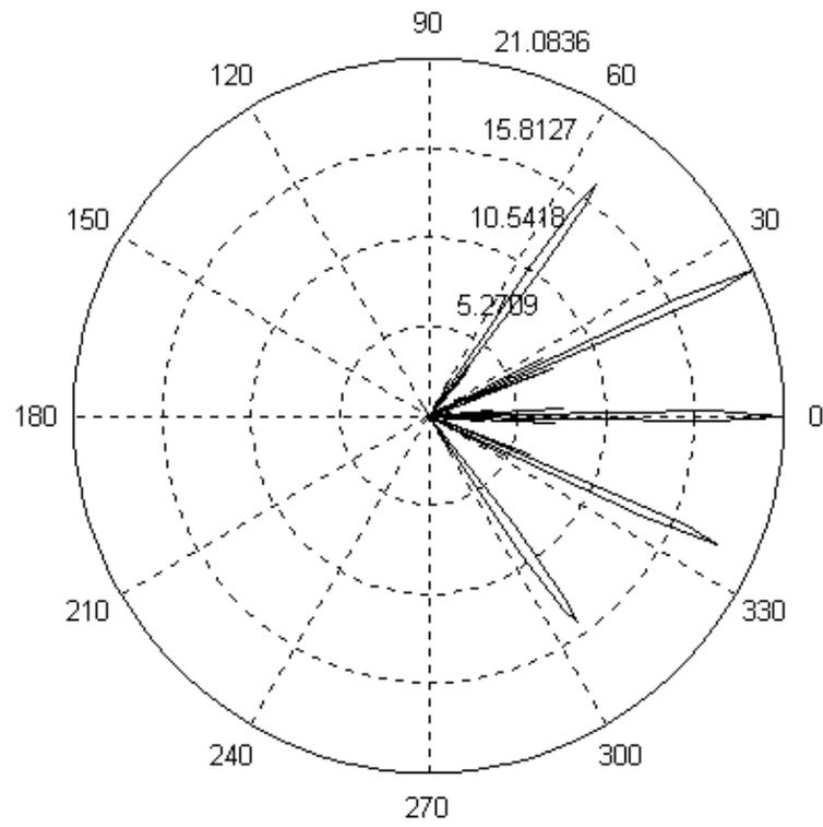
FIG. 3. Array of 12 speakers spaced at  $L = 2.5 \lambda$ .
