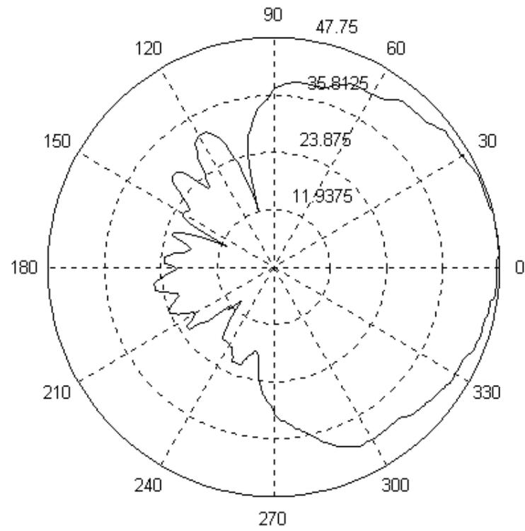
FIG. 2. Angular beam pattern for a single speaker.
