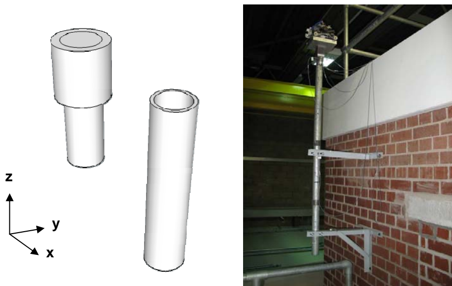
Figure 4: Left – illustration of the interface between turbine pivot shaft and mounting pole with axes for orientation. Right – a photograph of the laboratory test used to validate the method.
