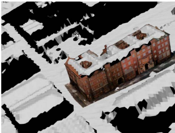
Figure 2: Merged LiDAR and Ground Based Scans of Jactin House, Salford, by Salford University
