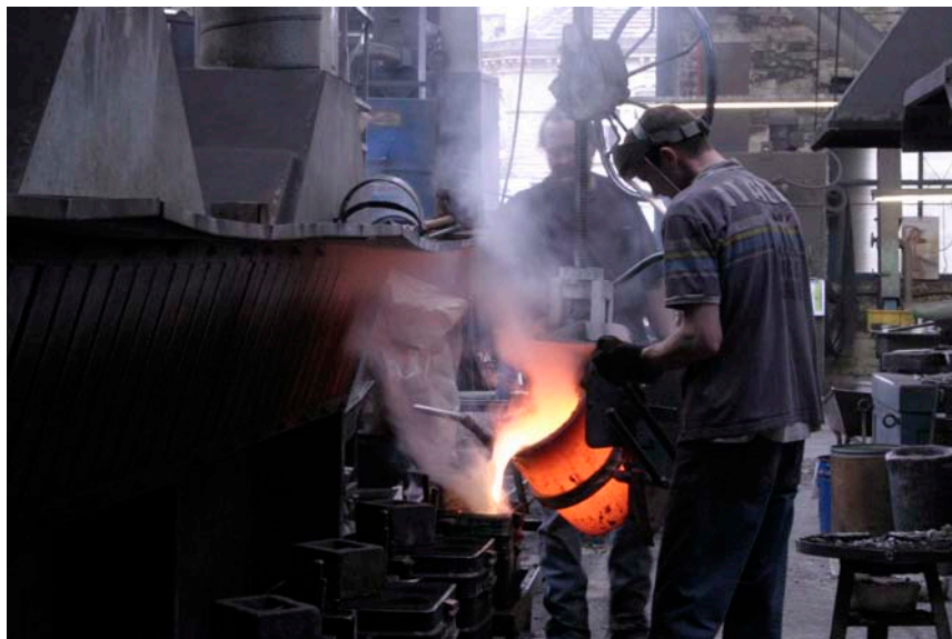
Pouring molten gun metal into the green sand moulds
