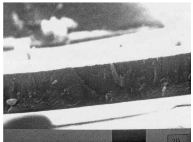
7 SEM micrograph of fracture section of CIS coating deposited onto glass substrate by PMS from CIS powder target
