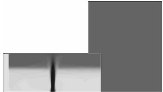
Figure 8. CFD prediction showing the temperature distribution in the single storey and the atrium (darker regions denote warmer air)
