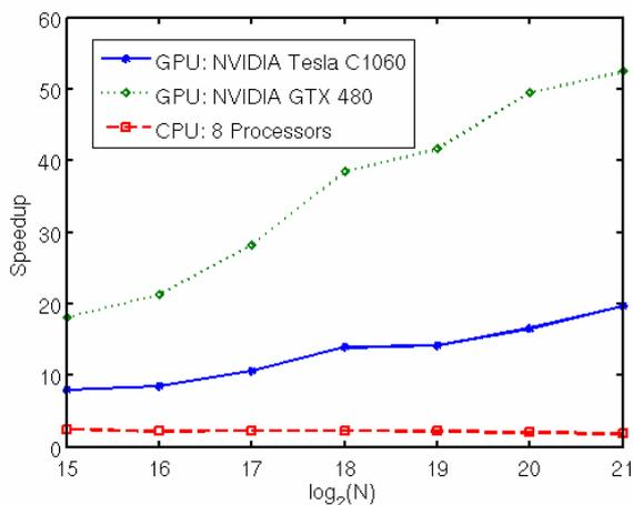
Fig. 4. Measured speedup relative to the one-processor execution for double precision floating point calculation as a function of the number of data points.
