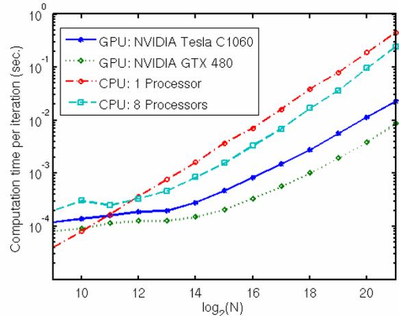
Fig. 2. Logarithmic plot of the floating point double precision computation time for one step of the numerical scheme calculated on a run of ten thousand iterations.
