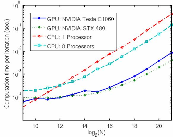
Fig. 1. Logarithmic plot of the floating pointing single precision computation time for one step of the numerical scheme calculated on a run of ten thousand iterations.
