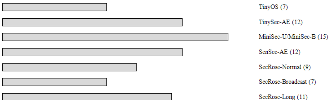
Fig. 3. Comparison of packet overhead of all proposed solutions. Numbers in parenthesis indicate the size in bytes.
