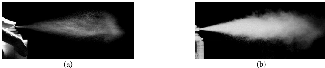
Figure 9: Spray pulses from (upper photograph) new metered valve using water (compressed air propellant), and (lower photograph) commercial freshmatic air-freshener with conventional liquefied gas valve (mainly butane propellant).
