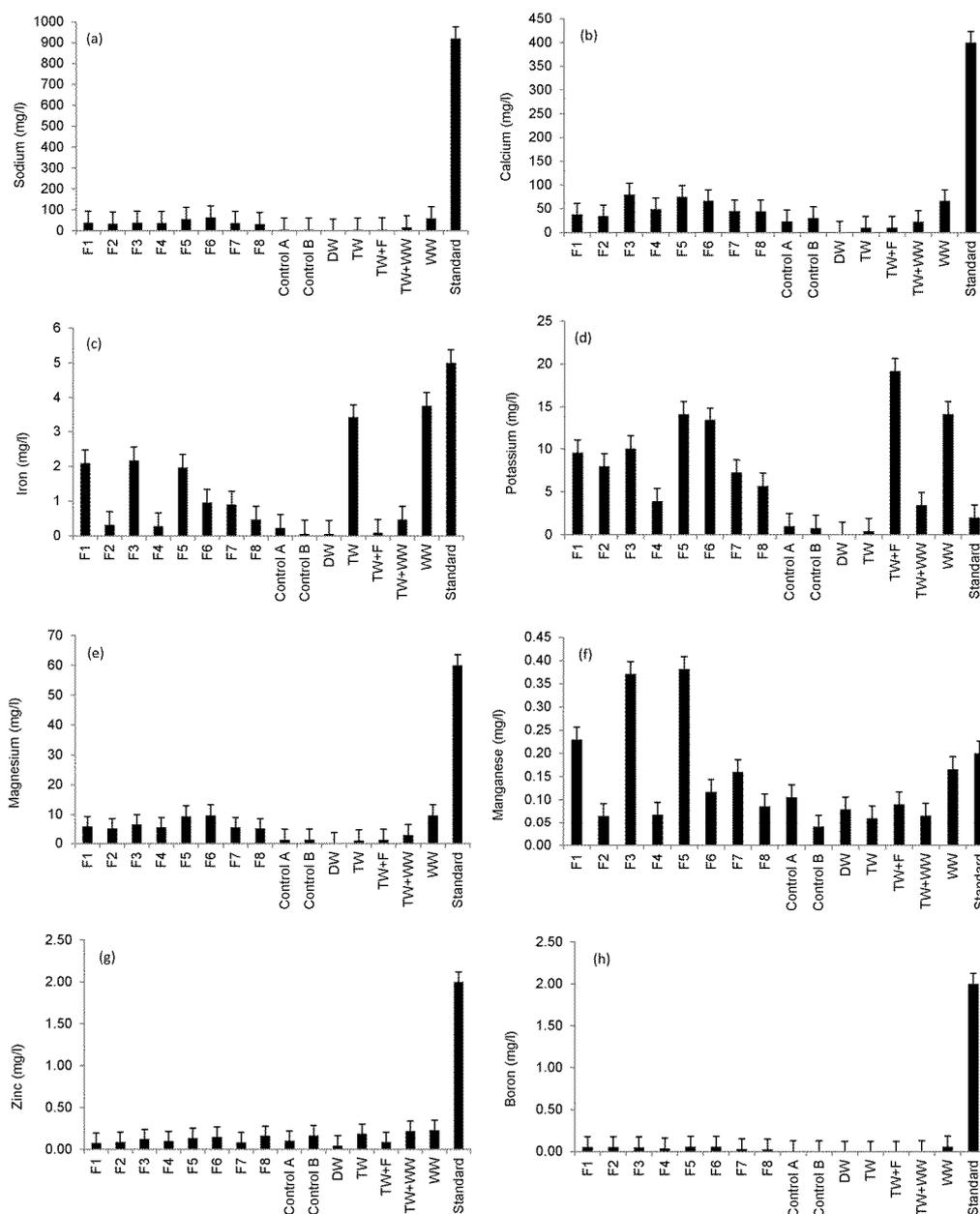
**Figure 1.** Overview of the Inductively Coupled Plasma—Optical Emission Spectrometer (ICP—OES) analysis (sample number: 10; 11 October 2013 to 25 September 2014) for detected elements compared with common standards for irrigation water [25,27].
