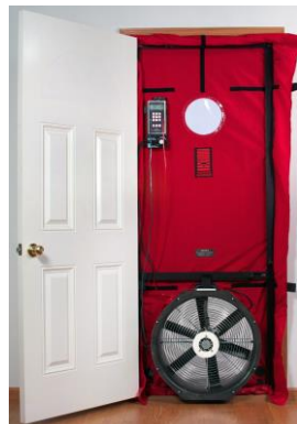
Figure 4: Air tightness test
