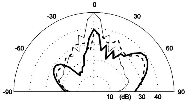
Fig. 19. The predicted scattering from three surfaces for the 1kHz 1/3 octave band.
