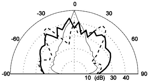
Fig. 10. Predicted scattering from three surfaces for 2kHz 1/3 octave band.
