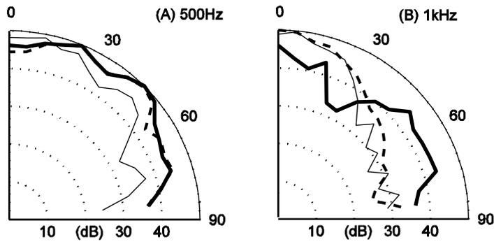
Fig. 6. Measured scattering from three surfaces at two different frequencies.
