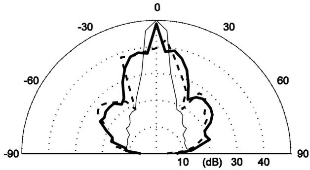
Fig. 18. The predicted scattering from three surfaces for the 315Hz 1/3 octave band.
