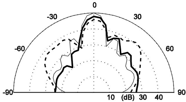
Fig. 9. Predicted scattering from three surfaces for 500Hz 1/3 octave band.
