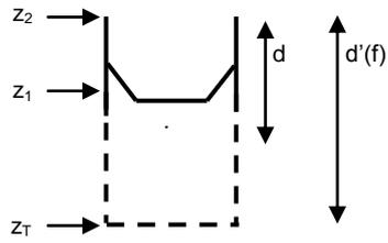
Fig. 5. Filter functions to achieve a pressure reflection coefficient of -1 at the well entrance:
