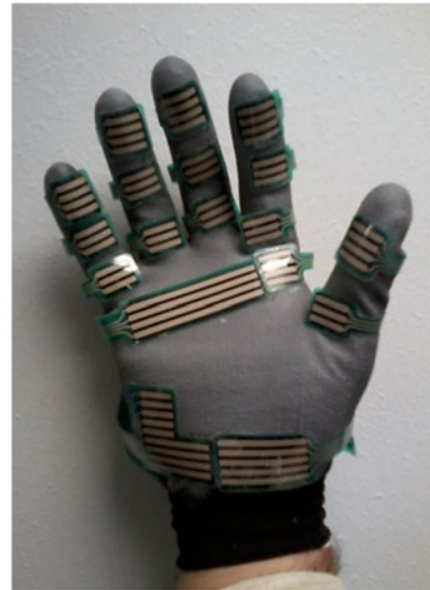
Fig. 1 Position of the sensors on the force sensing glove
