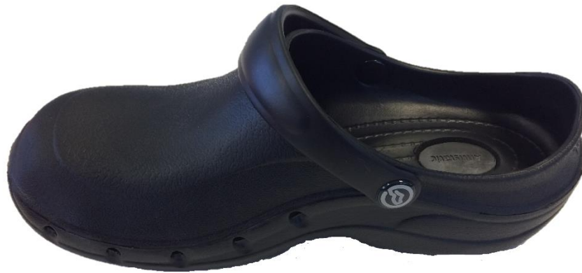
Figure 1: EVA shoe used for testing (Eziklog, Toffeln Ltd, UK). Both shoes had identical geometry but were made in material that the manufacturers deemed different in manual feel.
