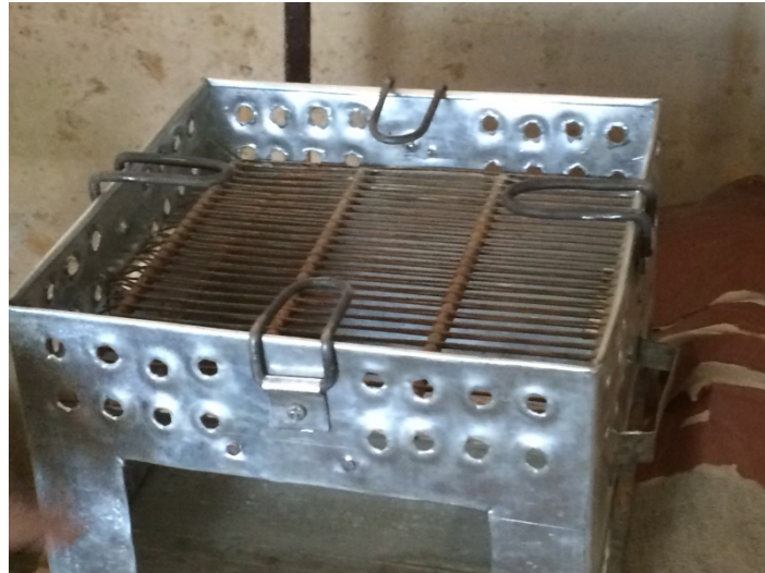
Figure 3. Coal Stove Made from Combination of Salvaged Roofing Sheets
