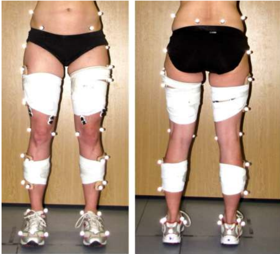
171 Figure 1: The placement of the markers and the sEMG electrodes
