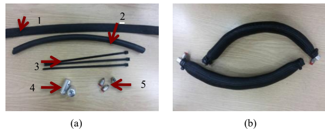
Figure 2. a) pMA components: 1. Braided mesh, 2. Inner tube, 3. Cable ties, 4. End caps, 5. Air inlet, b) pMA Build-up
