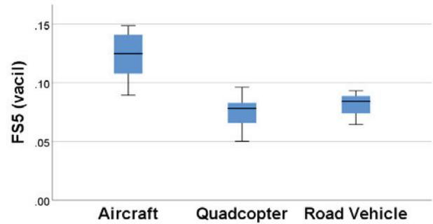
**Figure 4.** Distribution of 5<sup>th</sup> percentiles of Fluctuation Strength values for each vehicle category.
