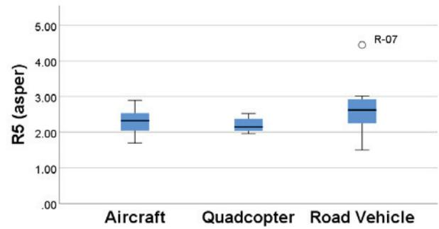
**Figure 3.** Distribution of 5<sup>th</sup> percentiles of Roughness values for each vehicle category.
