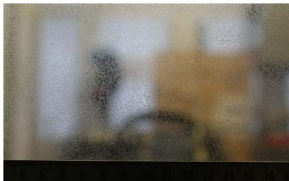
Figure 11. Impacted droplet deposition on glass test surface using sweeping action at the application distance of 1600mm ( L/D=6 )
