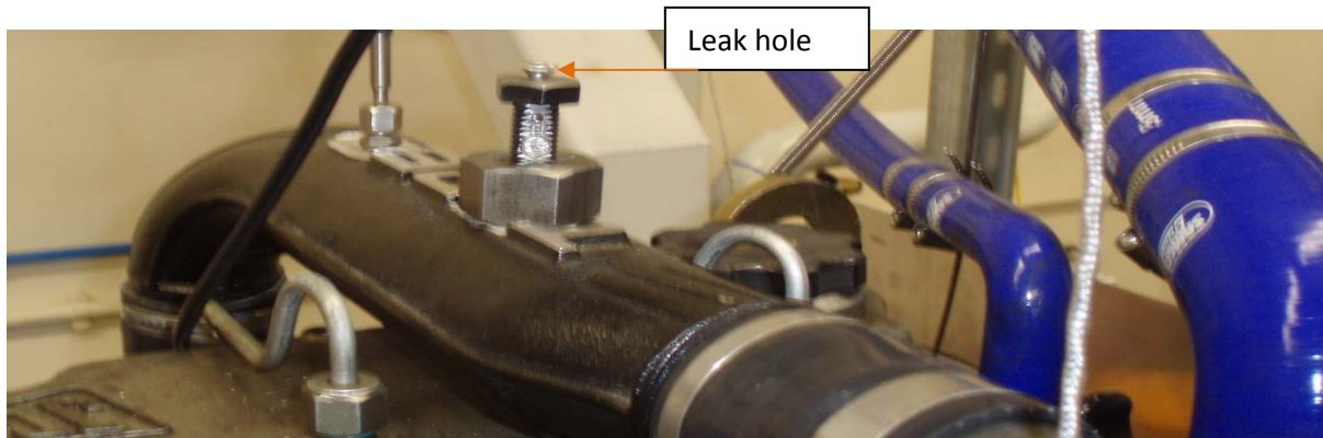
Figure 3 - Leak hole location on the outlet of turbocharger compressor
