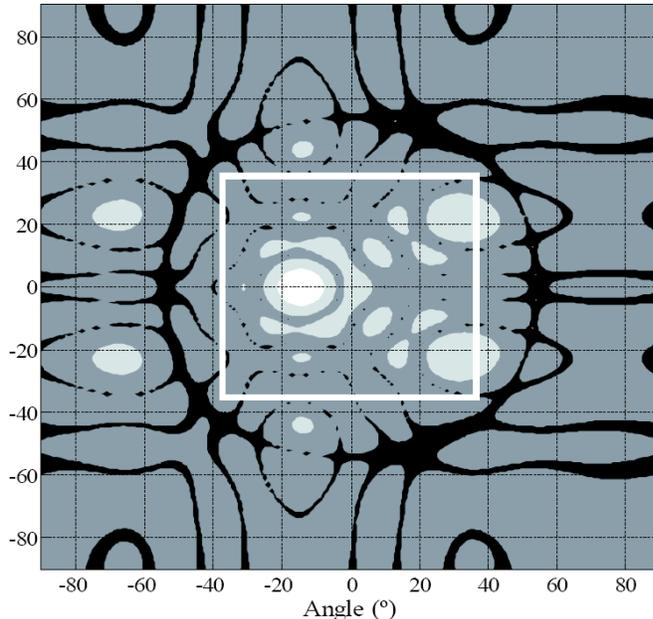
**Figure 3.1** Beam pattern calculated at top edge of the acoustic shield to indicate side lobe diffraction over the baffle edge. Bright colours denote high acoustic intensities that would potentially cause fixed echoes in beam direction. These will be particularly strong when intersecting the Sodar baffles.
