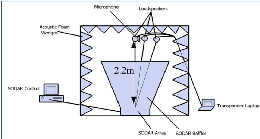
**Figure 3.3** Transponder setup in semianechoic chamber Note that the extended transponder transmits sound from three different directions.
