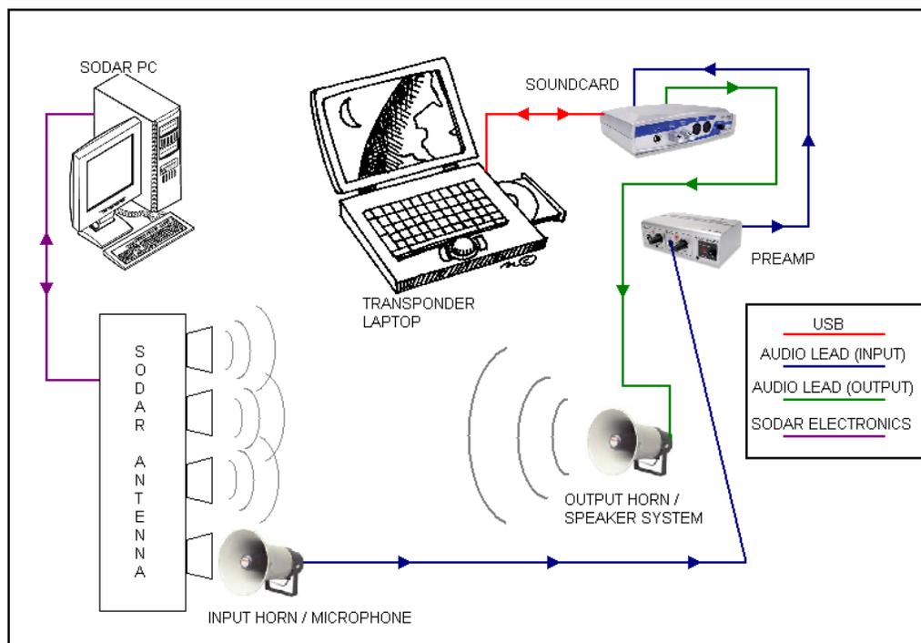
**Figure 3.2 Simplified transponder schematic. The SODAR consist of the Sodar antenna and PC whereas the transponder consists of a microphone with preamplifier, loudspeaker and laptop with an external soundcard.**
