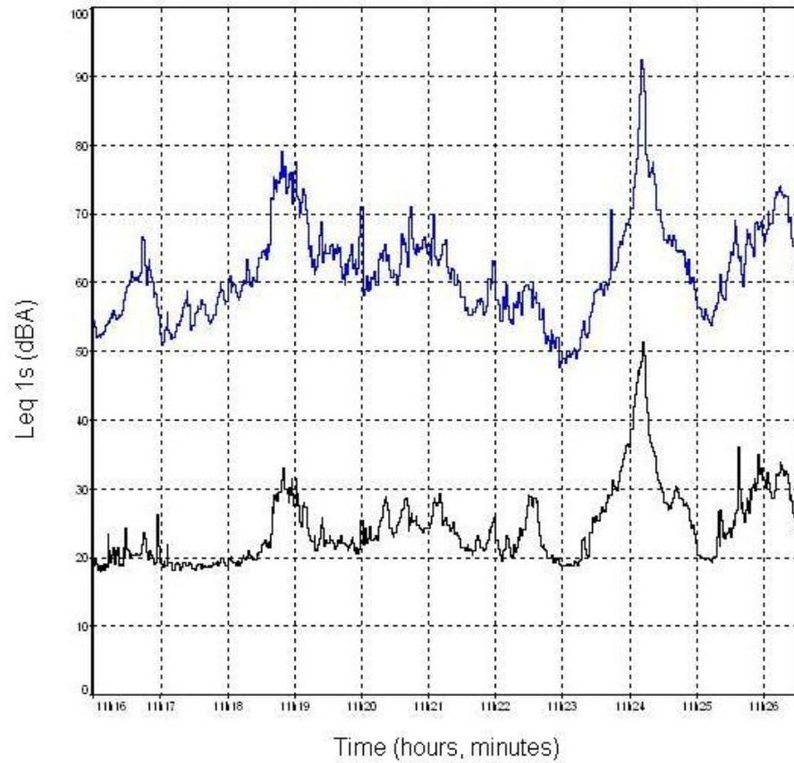
**Figure 3: Leq dBA level time histories measured inside and outside the front left bedroom. High level trial flyby used for insulation calculations: 11h24m08 to 11h24m14. Routine operational flyby: 11h16m36 to 11h16m52**
