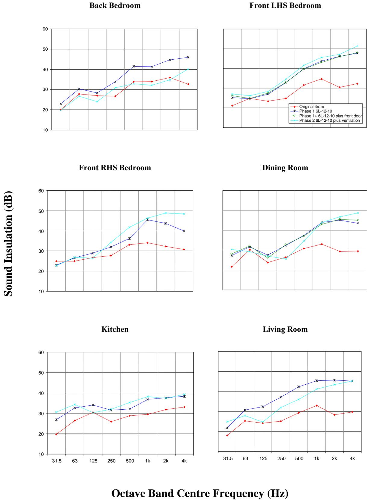
Figure 5: Sound insulation measured in each room
