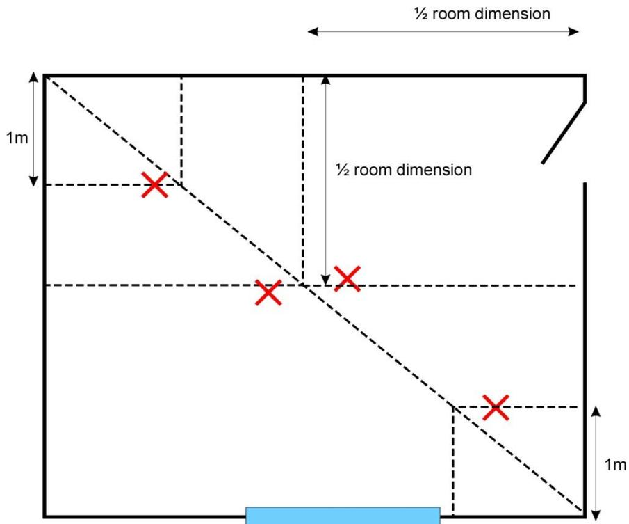
**Figure 2 Typical microphone positions**
