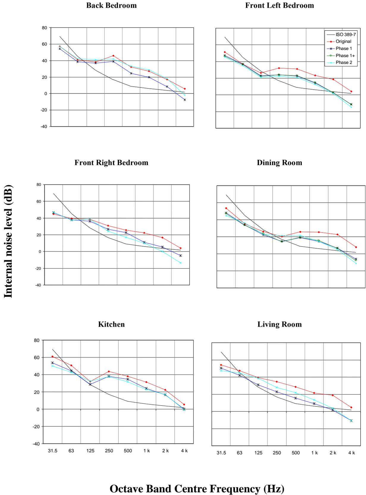
Figure 6: Internal noise level measured in each room
