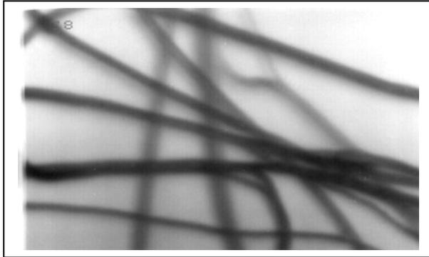
Fig 2. A SEM image of a sample, which shows clearly the size of the SWNT, bundles in the sample. As can be seen the diameter of the bundles
