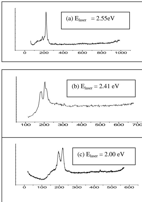
Fig 5. Raman spectra of the Radial Breathing Mode (RBM) of single wall carbon nanotubes with three laser lines.
