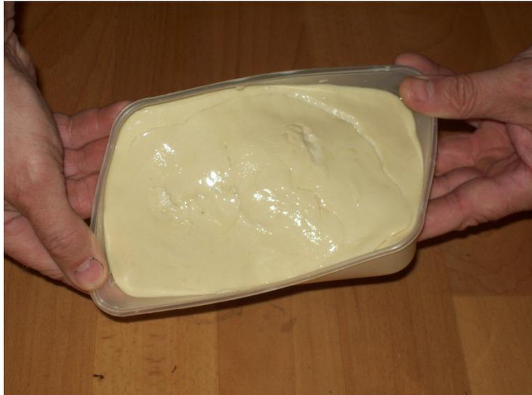
Fig.2: This waste engine oil soap remained in a “blancmange” state. (Read, 2012)
