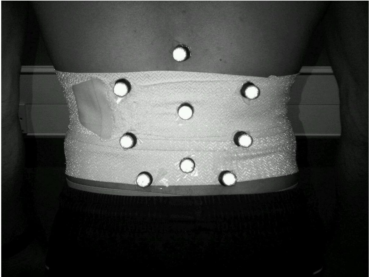
Figure 1a: Image of the marker set used to track the lumbar spine during running
