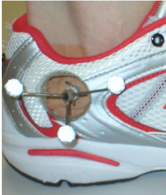
Figure 3: Three markers mounted on a metal triad, attached to the lateral heel via an aperture in the heel counter threaded onto a rigid plastic base that was taped to the lateral heel.
