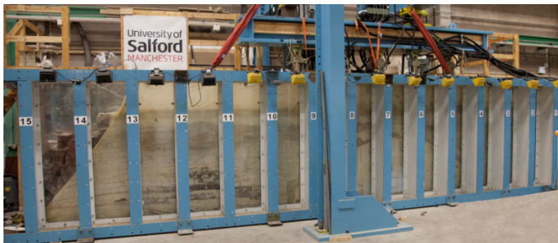
Fig. 2. Masonry arch bridge test chamber located at the University of Salford.
