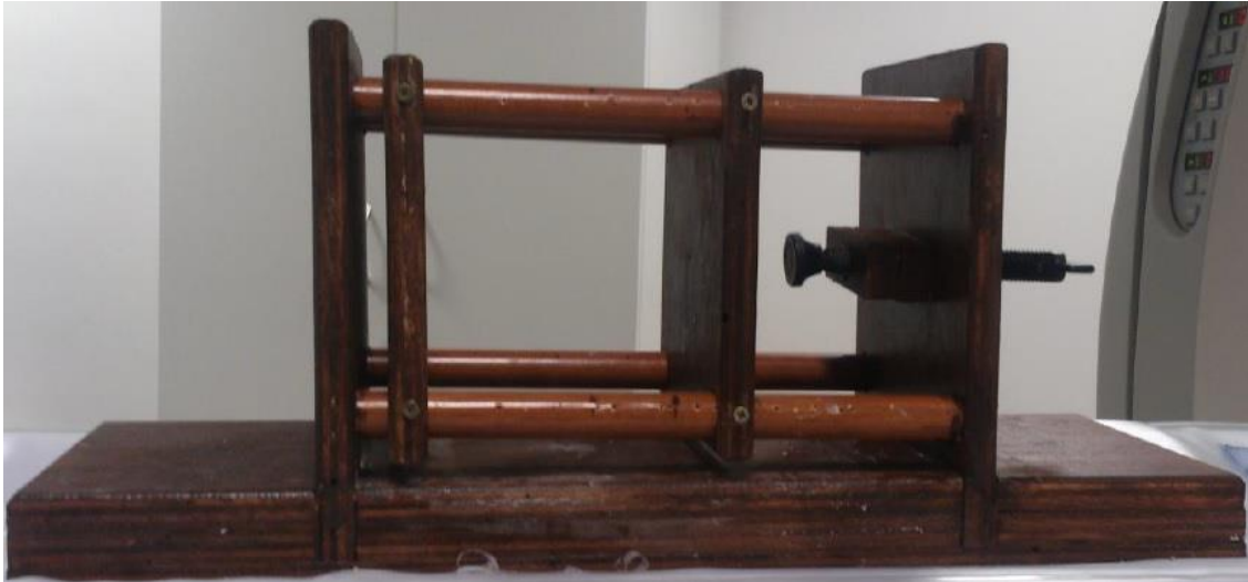
Figure 2: The custom-made jig that enabled phantom thickness reduction on the CT table.
