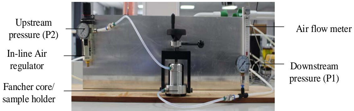
Figure 3: Set up for gas permeability determination
