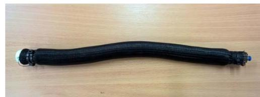
Figure.1 The photograph of the 32 cm extensor PMA
