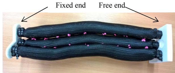
Figure.12 Four 30 cm extensor PMA's continuum arm
