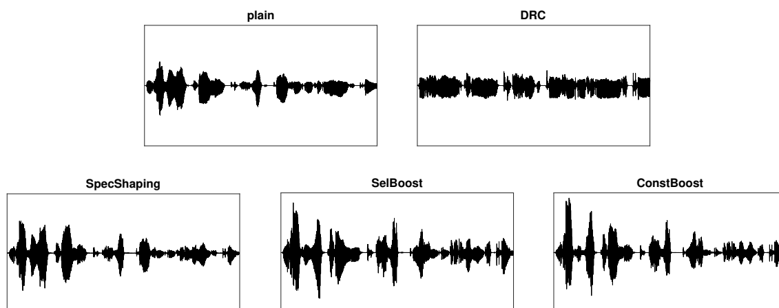
Figure 2. Waveforms of unmodified and modified utterance of ‘The overweight charmer could slip poison into anyone’s tea’.
