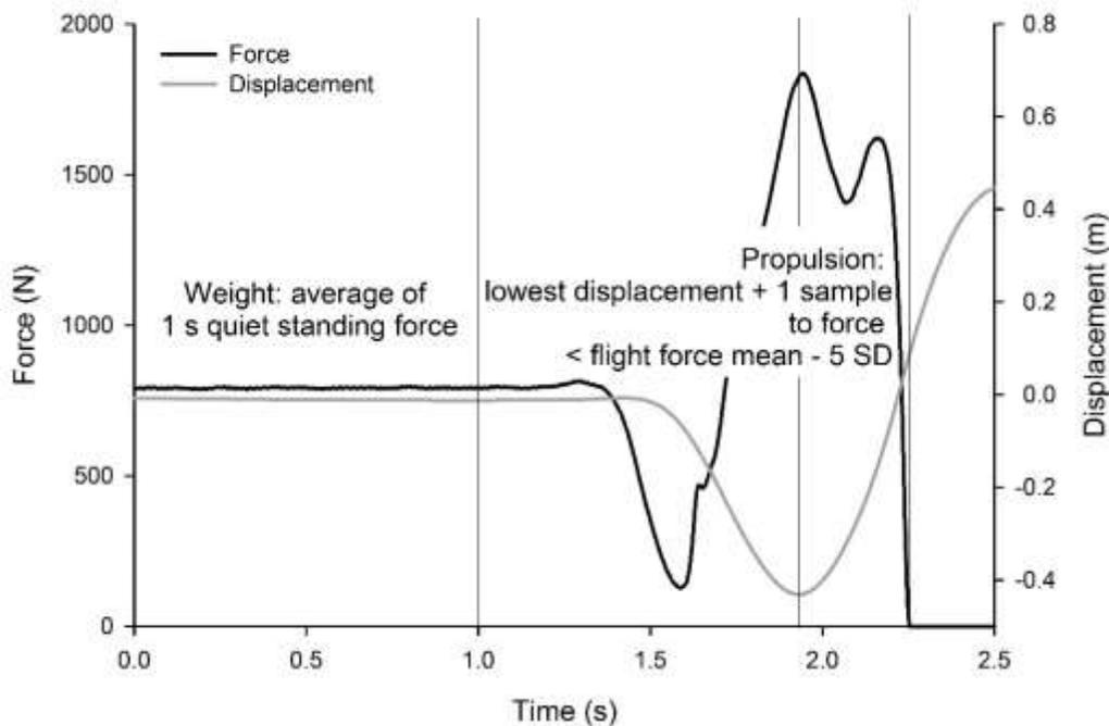
Figure 1. Calculation of weight and identification of the propulsion phase.
