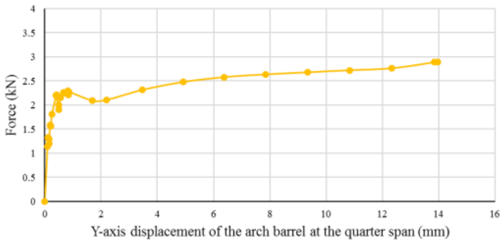
Figure 5: Load – displacement of arch on fixed abutments.
