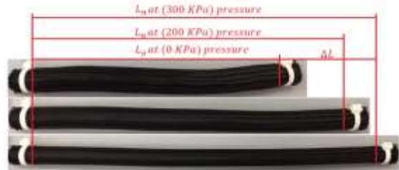
Figure 4. The extensor muscle with different supplied pressures, where:  $L_0$  is the muscle length at the rest,  $L_n$  is the muscle length under pressurization and  $\Delta L$  is the amount of length increase.
