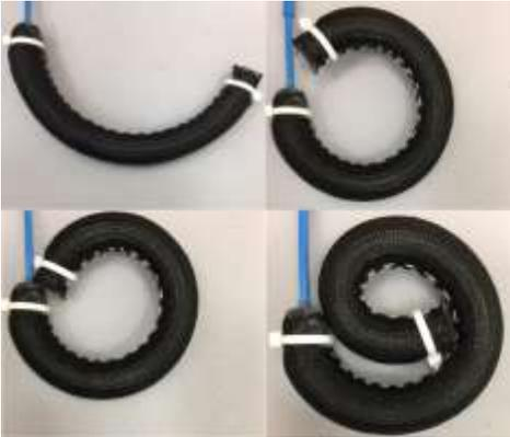
Figure 6. The bending artificial muscle with different pressures.
