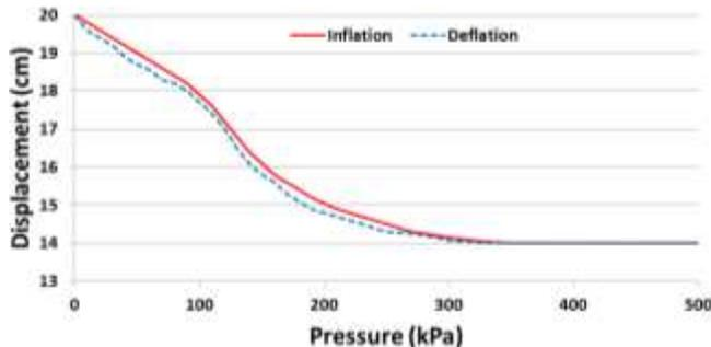
Figure 2. Measured muscle contraction with the applied pressure.
