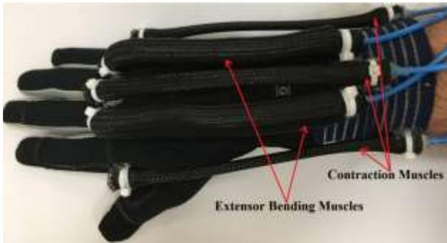
Figure 13. The proposed wrist soft exoskeleton.
