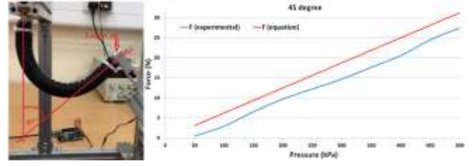
(a) The actuator in 45°bending angle.
