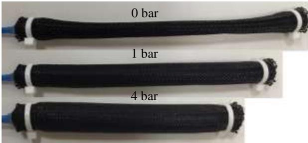
Figure 1. The contraction muscle with different pressures.
