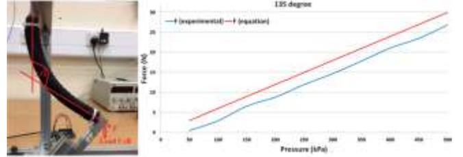
(c) The actuator in 135°bending angle.
