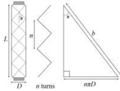
Figure 8. The general geometry of pneumatic artificial muscles.
