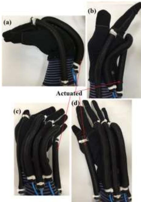
Figure 14. The rehabilitation movements of the proposed wrist soft exoskeleton; (a) Wrist flexion movement, (b) Wrist extension movement, (c) Wrist ulnar deviation movement (d) Wrist radial deviation movement.
