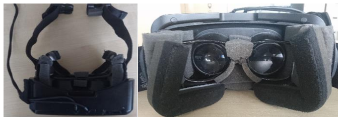
Fig.2. Oculus Rift DK2 adapted for fNIRS
