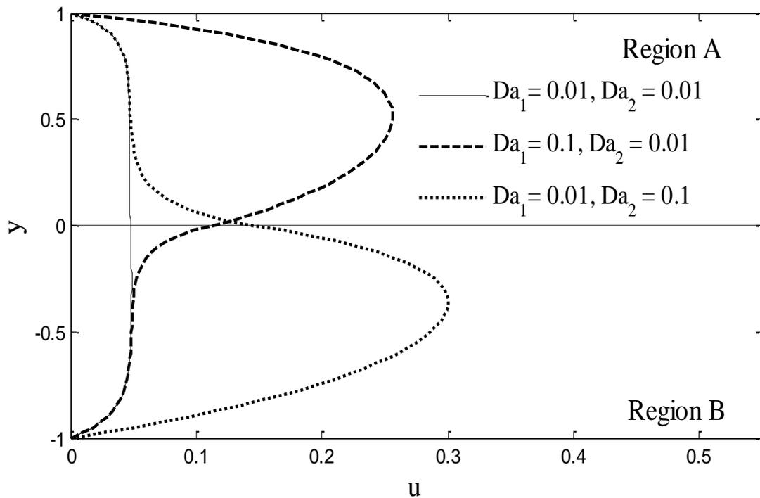
**Fig. 6.**  $y$  versus  $u$  i.e.  $u_1^*$  and  $u_2^*$  (both region A and B) for various  $Da_1$ ,  $Da_2$  [Darcy numbers for region A and region B] - for Darcian case only i.e.  $F_{s1} = F_{s2} = 0$ .
