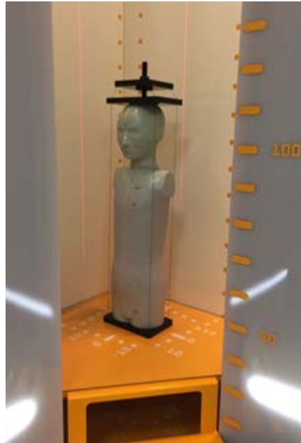
Figure 3: The phantom inside an EOS imaging system. The light on both sides shows the position of the X-ray tubes.
