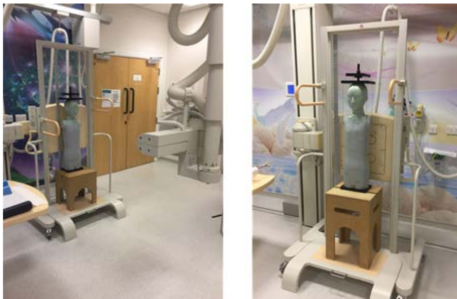
Figure 2: Shows the phantom while it is imaged using the conventional projection radiography imaging machines
