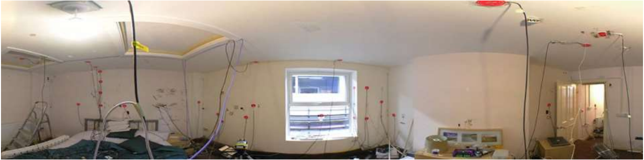
Figure 3 Heat flux and temperature sensors and their layout within the Energy House facility during the retrofit process
