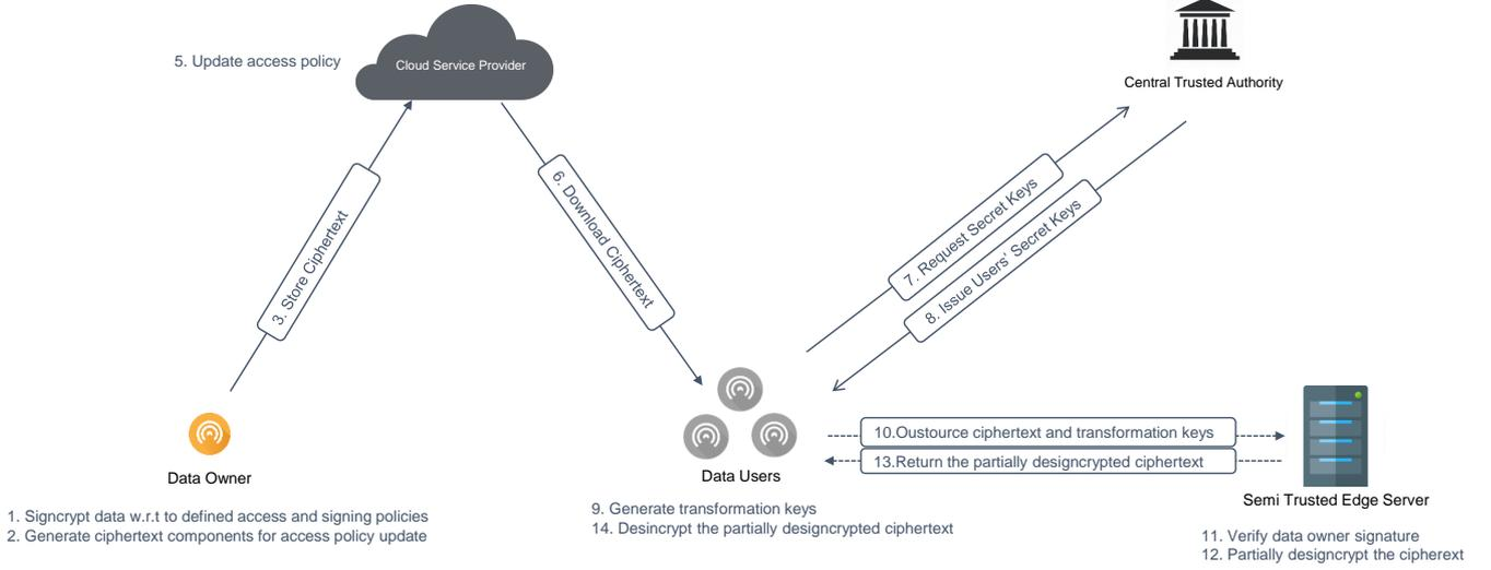
Figure 1: PROUD architecture and key interactions between different entities. The data owner takes advantage of cloud servers to share his data with a set of users, specifying access control policies and signcrypting the data. We consider data users to be resource-constrained IoT devices. The data users delegate a part of data designcrypting to edge servers, which is more powerful than the IoT devices.
