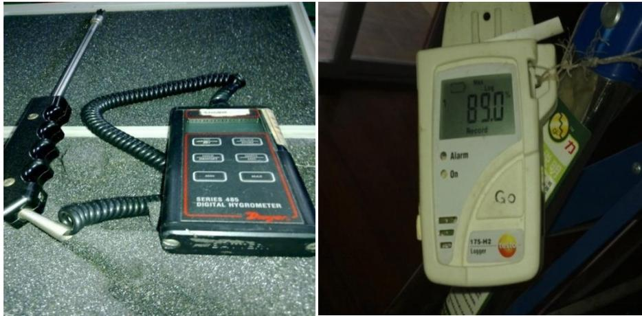
**Fig. 2.** Dwyer and Testo temperature and humidity recorder
