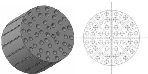
Figure 2. A porous sample with dead-ends (after sealing the circumference) used in the measurements. The sample diameter is 44.4 mm, and its thickness is  $L=30\text{ mm}$ .
