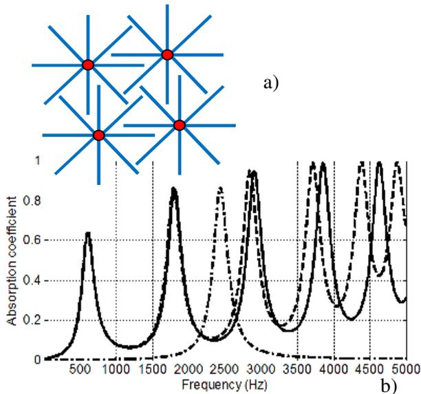
Figure 4. Example of possible design for the front face of a perforated material with lateral dead-ends and b) simulated results. In this example,  $N = 8$ ,  $a_{mp} = 2 \text{ mm}$ ,  $a_{de} = 1.5 \text{ mm}$ ,  $d = 1 \text{ cm}$ ,  $h = 3.5 \text{ mm}$ , slab thickness  $L = 3.5 \text{ cm}$ , perforation rate:  $\phi = 5.39 \%$ . Plain curve: low frequency approximation, dashed line: full model, dash-dot line: main pores without dead-ends..
