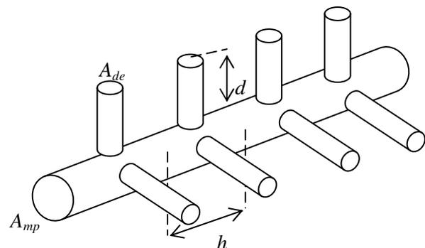
Figure 1. Main pore (cross sectional area  $A_{mp}$ ) with periodically arranged dead-end pores,  $N=2$  identical dead-end pores with cross section area  $A_{de}$  and length  $d$  per period  $h$ . The dead-ends are located at “nodes”.
