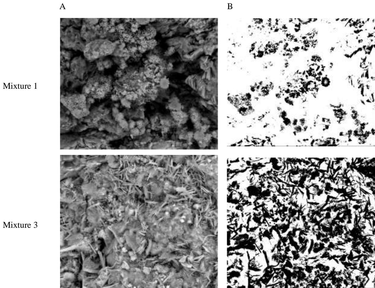
Figure 2-a. Image binarization for mixtures 1 and 3 at 7 days
