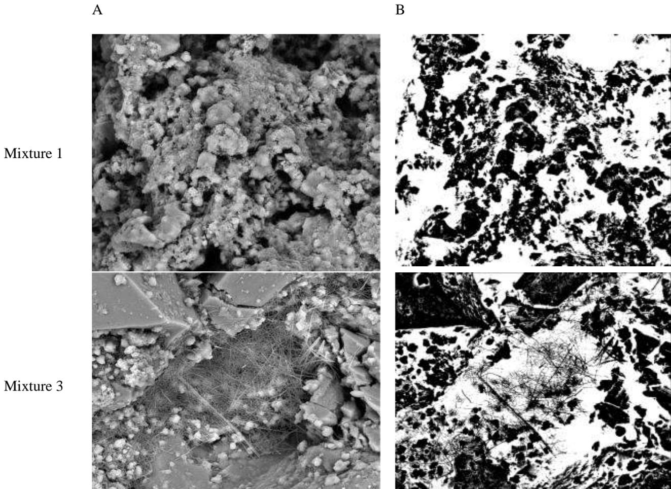
Figure 2-b. Image binarization for mixtures 1 and 3 at 28 days
