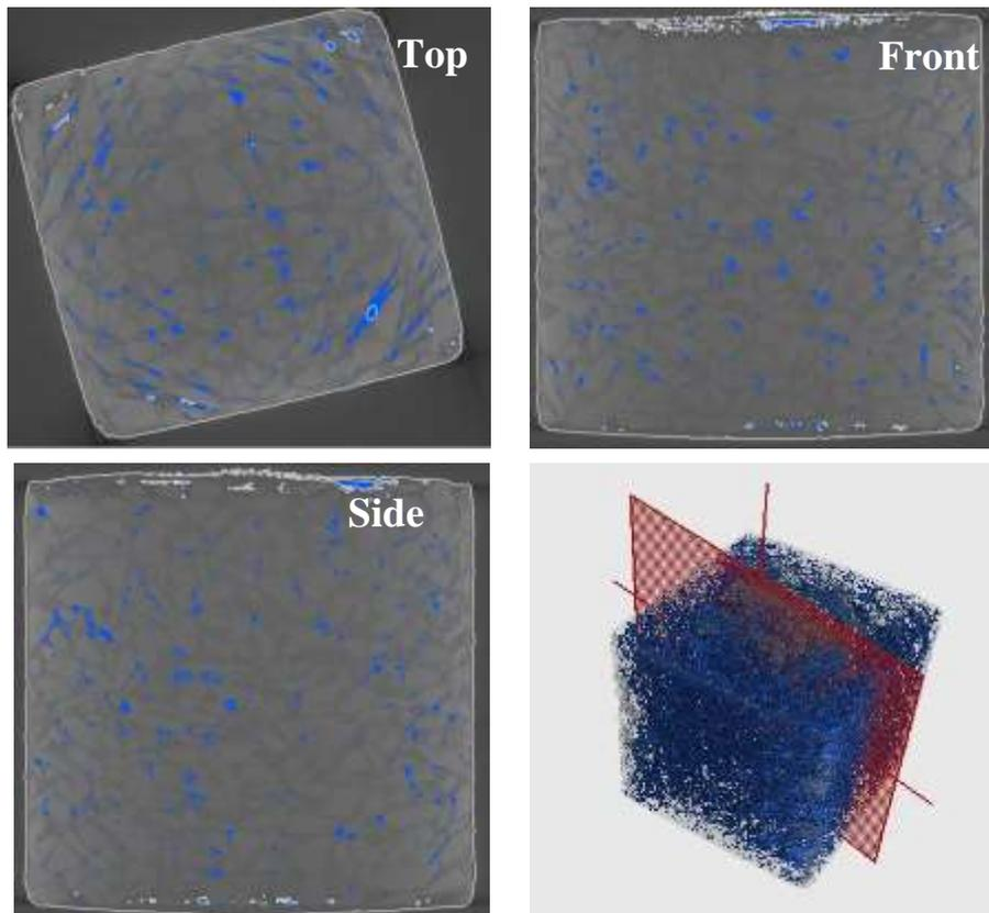
Figure 3. CT scan of mixture 1 concrete cube at age 56 days with 3D visualization of pores system in blue colour
