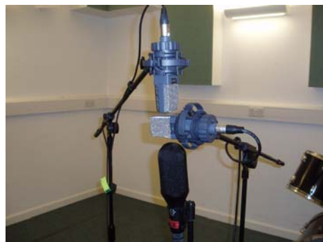
Figure 4 – Soundfield and Mid-Side arrangement for measurements in recording space. Soundfield microphone diaphragms are at 1.3 metres from the floor.
