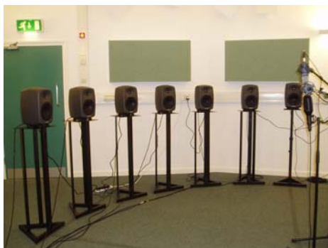
Figure 3 – Arrangement of 7 loudspeakers at a distance of 2 metres from microphones and ranging from 0° to 90° at 15° angles. Tweeter height is 1.3 metres.
